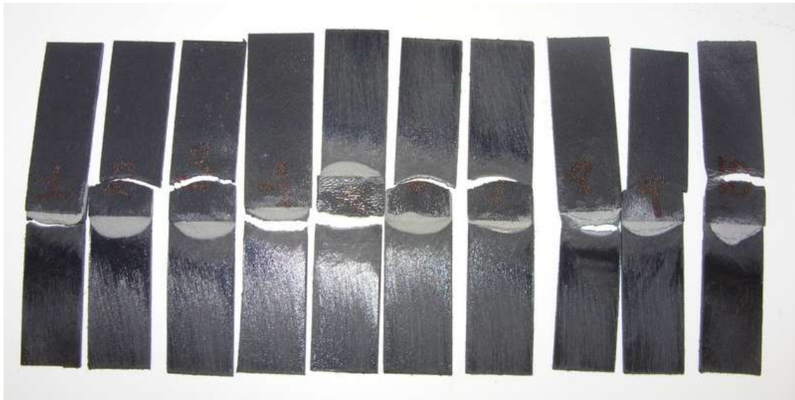
PHOTOGRAPH 3:- TEST PIECES – FAILURE MODE
